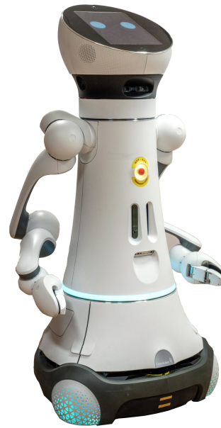
Figure 1. The assistive robot Care-O-Bot 4 configured with two arms and spherical hip and head joints.
