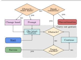
Fig. 4: Flowchart of a pointing gesture involving a spatial prompting mechanism. To reach its goal, the robot checks whether a potentially occupied area can be made accessible with the help of social signals to reach its goal. The gesture is only aborted if a defined exit condition is fulfilled.
